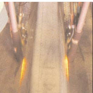
Automated submerged arc welder provides continuously welded joints
