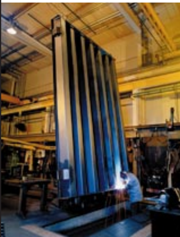
Module positioner allows all welds to be placed in the flat position
